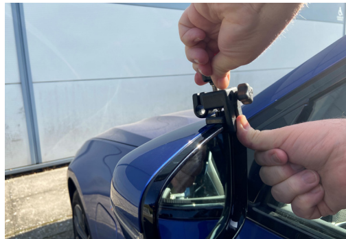
2. Fit the first mirror clamp, ensuring the wedge is fully inserted into the gap between the mirror and the wing mirror housing. Whilst holding the clamp firmly in place, turn screw 1 until the clamp is securely fitted.
