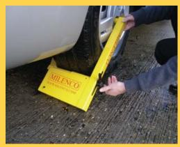
Turn winding handle to tighten up
