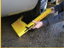
Turn the winding handle to widen the wheelclamp. Position wheelclamp into the wheelnut (use the enclosed wheelnut adaptors if required)
